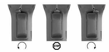
▶ Set the forward / reverse selector switch to forward or reverse rotation.
