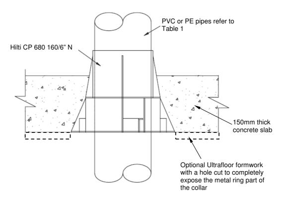
Figure 1 – Stack pipes protected with Hilti CP 160/6" N with or without Ultrafloor
