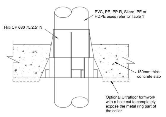
Figure 1 – Stack pipes protected with Hilti CP 75/2.5" N with or without Ultrafloor
