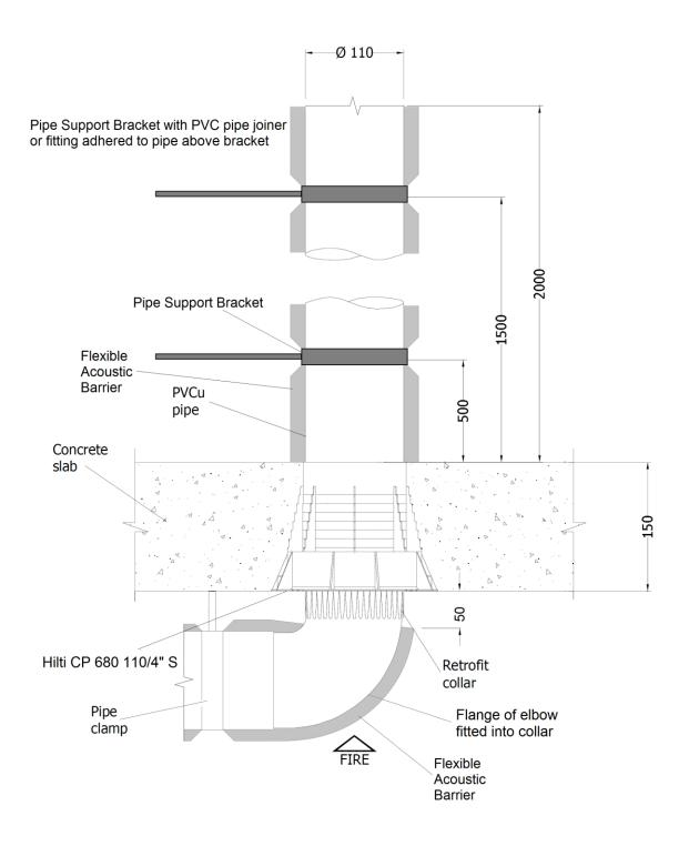
Figure 4 – uPVC pipes flange of elbow fitted into firestop collar protected with Hilti CP 680 10/4" S + CP 680 N-RAD Cast-In Firestop Collar System without Ultrafloor, optional flexible acoustic barrier at least 50mm from underside of concrete slab
