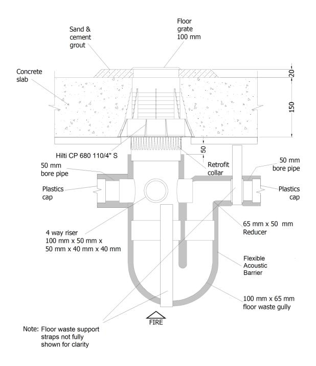
**Figure 7 –** uPVC floor waste – gully pipe protected with Hilti CP 680 110/4" S and Hilti CP 680 110/4" N-RAD with Ultrafloor, optional flexible acoustic barrier at least 50mm from underside of Ultrafloor
