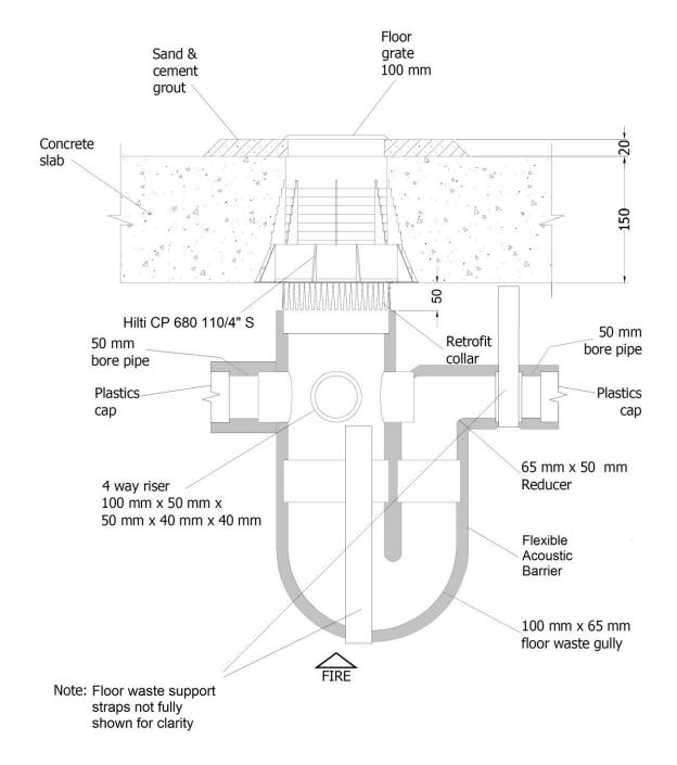
**Figure 8 –** uPVC floor waste – gully pipe protected with Hilti CP 680 110/4" S and Hilti CP 680 110/4" N-RAD without Ultrafloor, optional flexible acoustic barrier at least 50mm from underside of concrete slab
