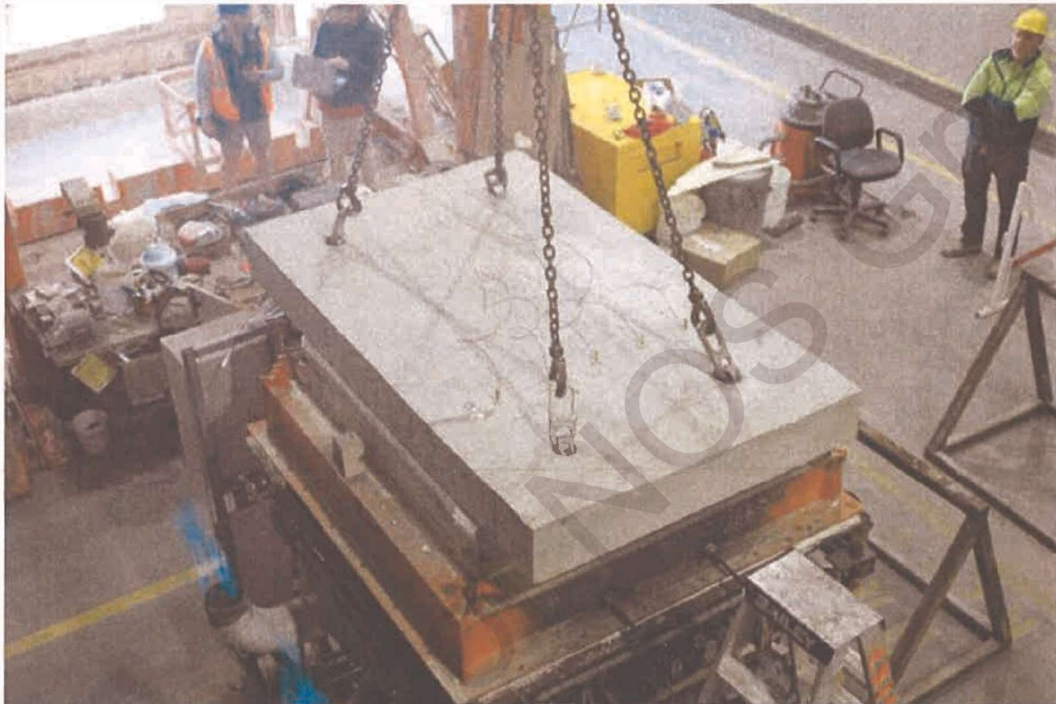
PHOTOGRAPH 9—SPECIMEN SET-UP AT THE CONCLUSION OF TESTING
