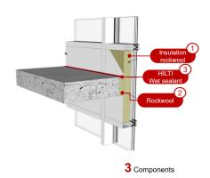
Joint between curtain wall with Steel or Aluminium framing, and rigid floor slab.
