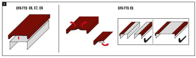
Fit CFS-TTS E6, E7 or E9 onto the top track
