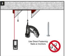
Fasten the top track with the CFS-TTS to the underside of the slab. Ensure surfaces are clean and dry.
