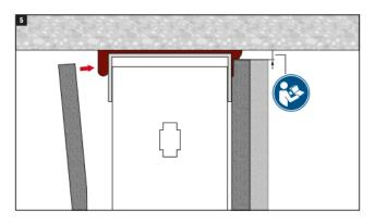
Install fire-rated plasterboard lining according to the plasterboard manufacturer's recommendations.
