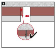
When joining two pieces of CFS-TTS together, a length of 15mm must be compressed at the joint as shown. This applies to CFS-TTS on separate tracks or on the same track.
