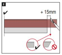
Cut the CFS-TTS such that there is an extra 15mm from both ends of the track
