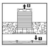
Remove the formwork, and the plastic cap.
