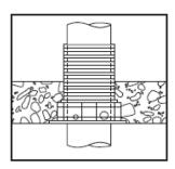
Slide the pipe into the CP 680 P/PX Cast-In Firestop Collar, and seal around the pipe using Hilti CP 606 Flexible Firestop Sealant as required in the approval documentation.
