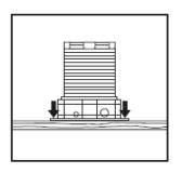
Place CP 680 P/PX Cast-In Firestop Collar in the desired position and fasten to the formwork.
