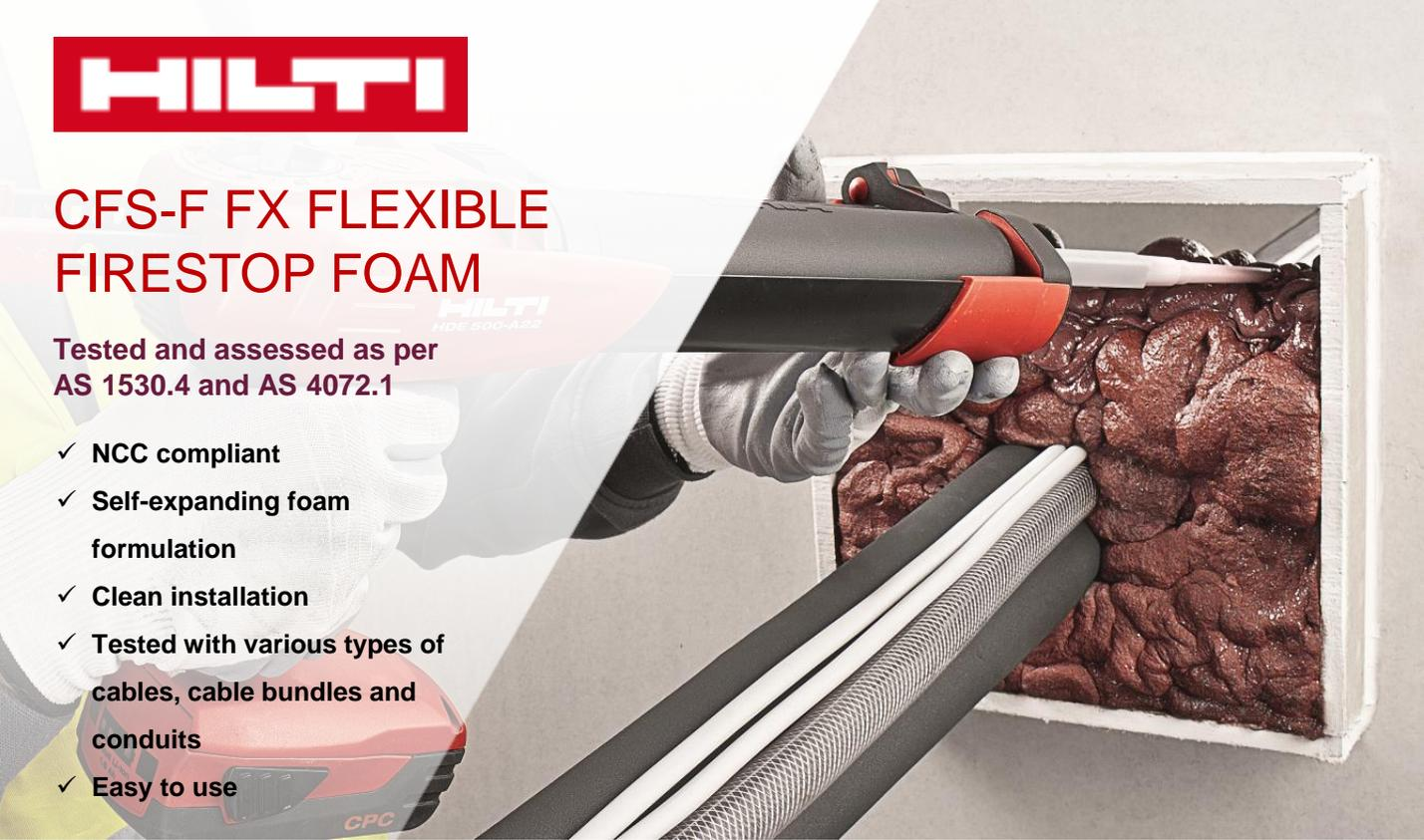
Hilti CFS-F FX Flexible Firestop Foam is a self-expanding, intumescent, two-component polyurethane foam that is ideal for sealing medium-sized holes and irregularly shaped openings in walls and floors. Hilti CFS-F FX is designed as a one-step solution for sealing around **cables, cable bundles and conduits** with or without cable trays to achieve an FRL of up to -/120/120. Hilti CFS-F FX Flexible Firestop Foam may be used with various base materials such as:
