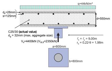
Punching shear resistance of non-reinforced slab (as evaluated by the applicable structural concrete code):
