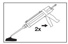
Fig. 26: Injection of dynamic set washer
