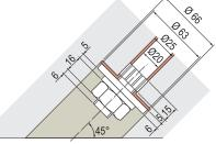
Fig. 24: Anchor head and hole extension HZA-P M16
