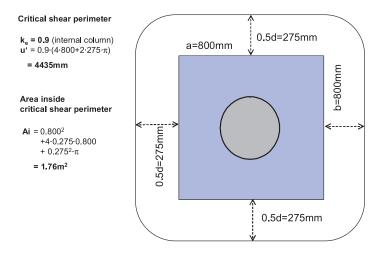
Punching shear load acting outside the critical shear perimeter:
