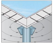
Fig. 6: post-installed punching shear reinforcement
