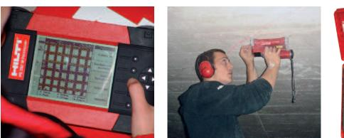
Fig. 20: location of reinforcement with Ferroscan PS 200
