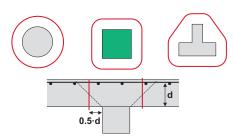
Fig. 12: shear perimeter u<sub>0</sub> for typical column shapes
