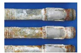
Zinc-coated carbon steel Zinc coated steel typically corrodes uniformly. Steel corrosion starts when the zinc protection is mostly consumed.
